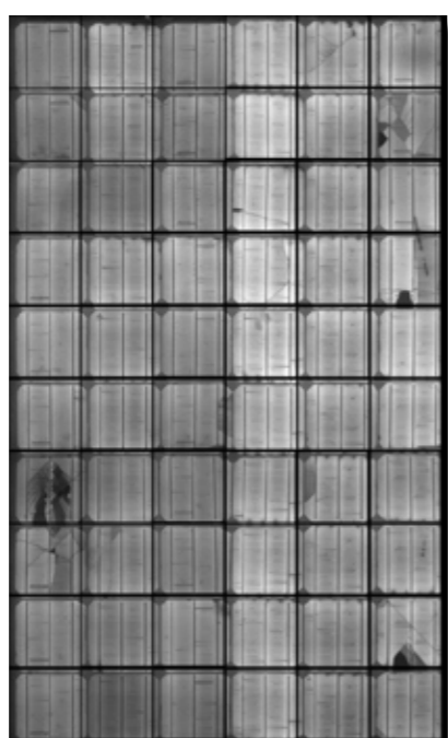
Defects found only with electroluminescence's test. Tests carried out on every module but not on random.
